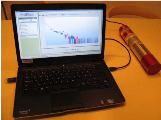
**Fig. 2:** A NaI-detector (scintillation detector) connected to an ordinary laptop. The detector is capable of measuring gamma photons from 20-2000 keV.
